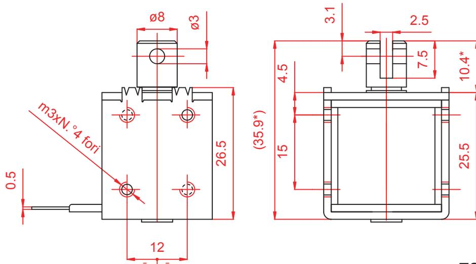
\* QUOTE CON ELETTROMAGNETE CHIUSO - CORSA = 0 mm
