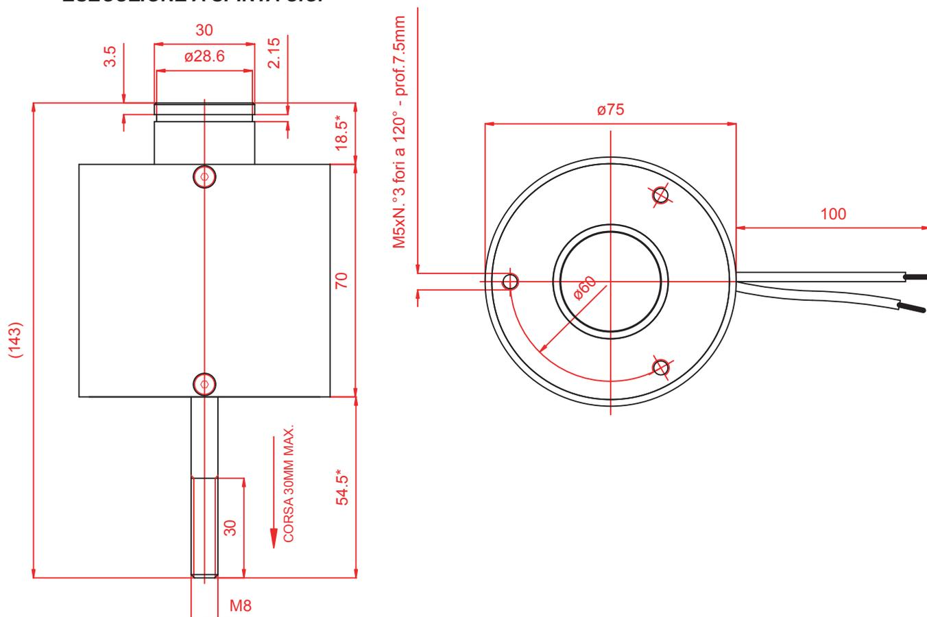
\* QUOTE CON ELETTROMAGNETE CHIUSO - CORSA = 0 mm
